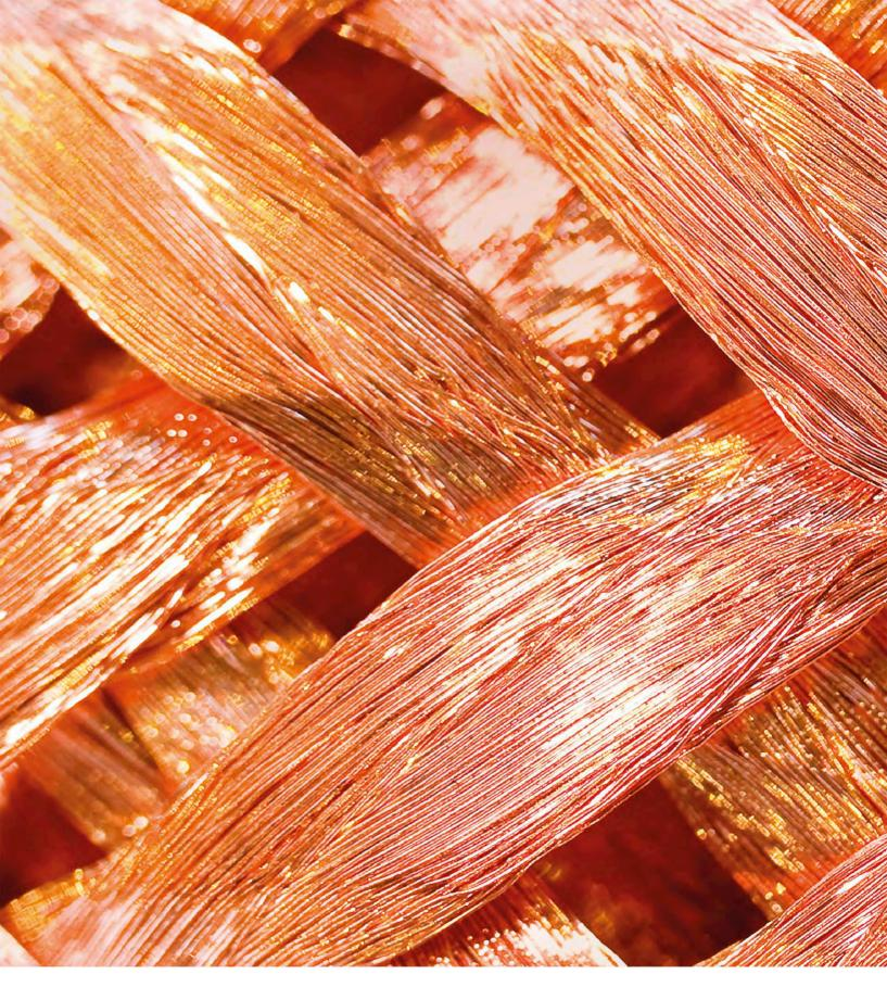
**COPPER WIRES** Not much thicker than a human hair, these copper wires are twisted together and woven into a tight bundle. One of the main uses for these wires is to shield a thicker copper wire that transmits a signal to a television. As the signal carries pictures and sounds in the form of electrical currents, the wires wrapped around it prevent interference from other electrical sources nearby.
