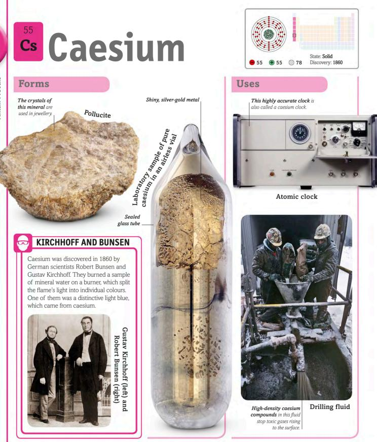
As the most reactive metal on Earth, caesium explodes into flames if in contact with air or water. Therefore, **pure caesium**, is stored in a sealed glass tube from which all the air has been sucked out. This element is rare, and most of it is extracted from the mineral **pollucite**. Its name
