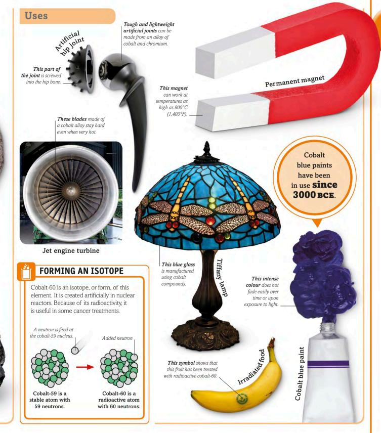
that can be used to make a permanent magnet. Large **permanent magnets** are made from a tough alloy of cobalt, nickel, and aluminium, called alnico. A radioactive form of cobalt, called cobalt-60, is produced in nuclear reactors. This form is widely employed to **irradiate food**, a process by which food is exposed to a tiny dose of radiation to kill harmful germs. Cobalt can also produce a deep shade of blue: **cobalt blue paints** and dyes are formed by reacting aluminium with cobalt oxide.
